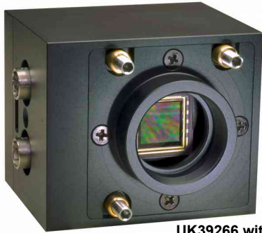
UK39266 with adjustment screws and C-mount adapter plate
